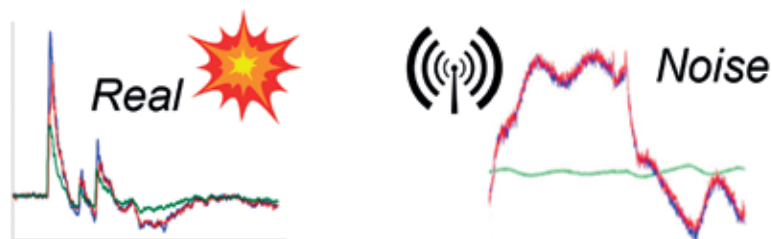
Figure 5: Illustrations of real blast (left) and noise signals (right) potentially recorded by person-borne blast dosimeters
