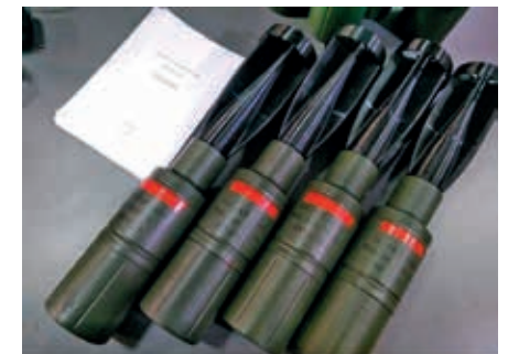
Picture 72. Modified RKG-3 anti-tank grenades with 3D-printed tail fins. 4
