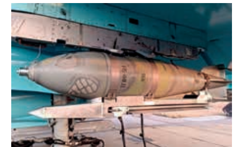
Picture 2. UMPC module on the FAB-500 aerial bomb 2
