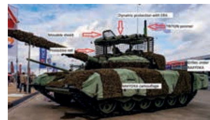
Picture 29. Factory-made protection mounted on T-72B3M tank 31
