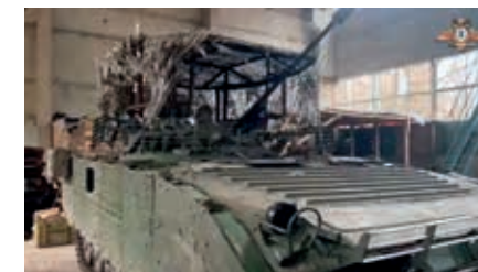
Picture 30. Improvised protection mounted on BMP-2 with factory-made additional space armour on vehicle sides
