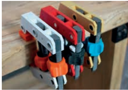
Picture 54. A set of 3D-printed clamps 25
