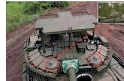
Picture 25. EW “Volnerez” mounted on tank T-80 BV 26
