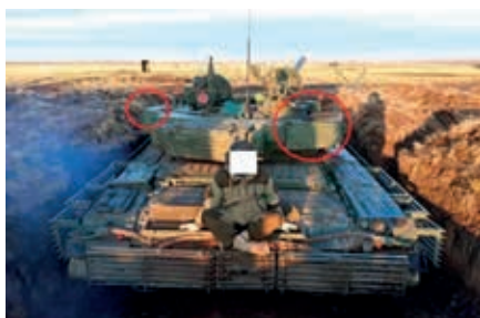
Picture 28. Arena-M mounted on T-72B3M tank 30
