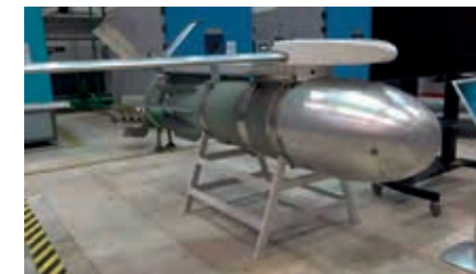
Russian FAB-1500-M54 aerial bomb with UMPK gliding and guidance kit (Photo source: https://armyrecognition.com/ )
