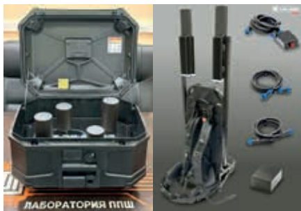
Picture 27. Left - Triton electronic warfare system for vehicle. Right - Triton electronic warfare system backpack 28
